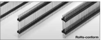
Materialtypical CuZn alloySurface2-3 µm nickel, 0,15 µm gold
